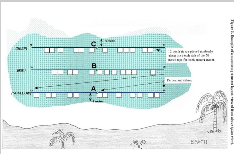
Figure 3. Example of a monitoring transect layout, viewed from above (plan view).
